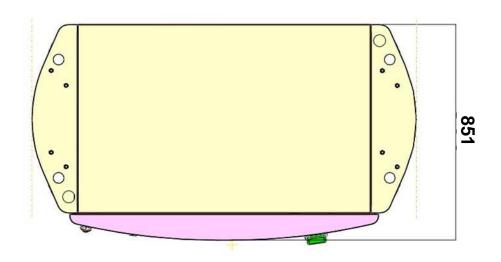
Stainless steel AISI-304 S.B. PP Thickness 1 & 1,5 mm
